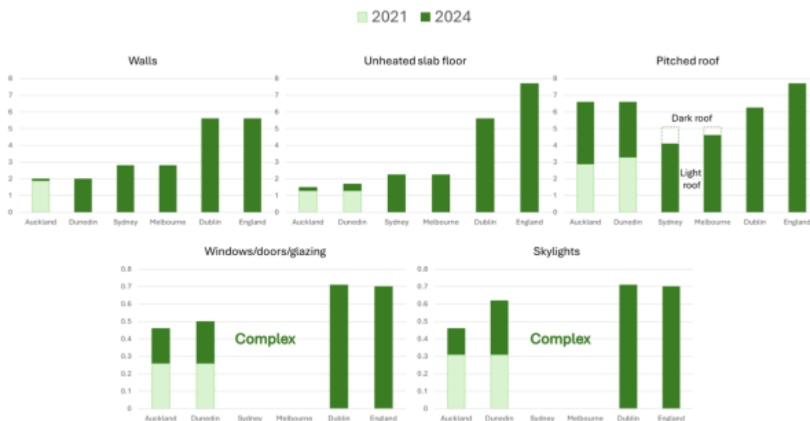
Figure 1. Minimum R-values (measure of how well a product prevents heat transfer) for different building elements in New Zealand and comparable climate locations.
